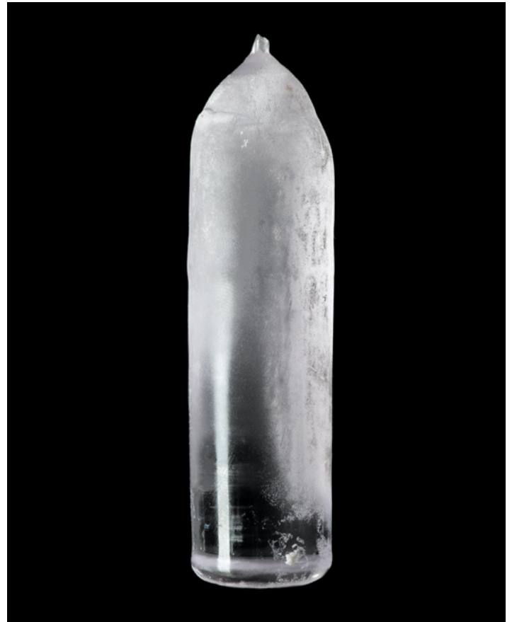
Fig. 1: Raw sapphire crystal grown with the Verneuil process
