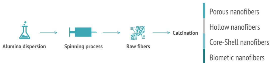
Figure 2: Diagram showing the broad production process for aluminous fibers.
