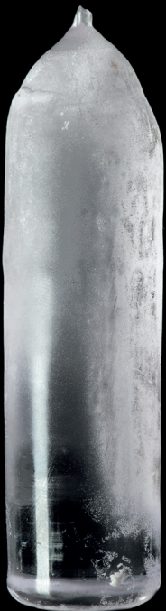
Fig. 1 Carrot produced in Verneuil process
